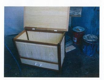
28. To spray my project I covered up all the hinges and handles. I then sprayed one coating with a lacquer then lightly sanded it back before spraying again. I completed this four times to give it a solid coating.
