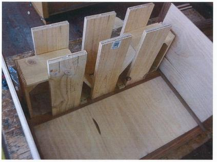
19. To ensure it all fitted I did a dry fit of the front with the sides.
