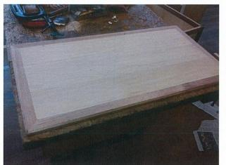
26. The edges were quite sharp so I decided to rout a 45 degree edge which was very simple as I used a router with a cutting bit with a bearing on it(no jig needed)
